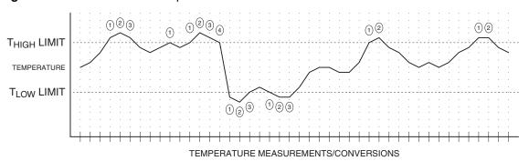
Figure 5-1. Fault Count Example
