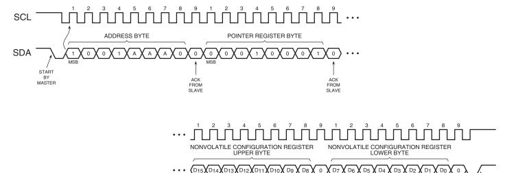
Figure 6-7. Read from Nonvolatile Configuration Register
