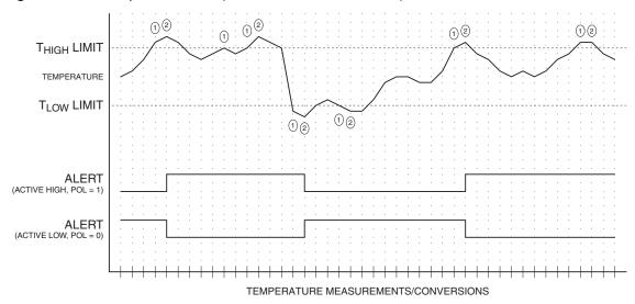
**Figure 5-2.** Comparator Mode (Fault Tolerance Queue = 2)
