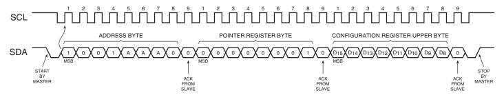
Figure 6-5. Read from Configuration Register
