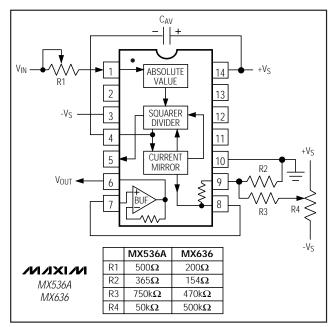
Figure 4. Optional External Gain and Output Offset Trims
