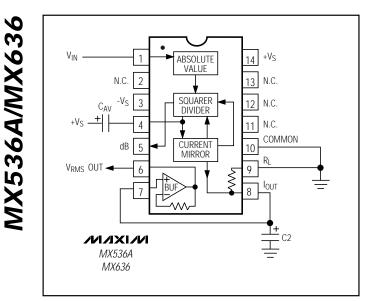
Figure 7. MX536A/MX636 with a One-Pole Output Filter
