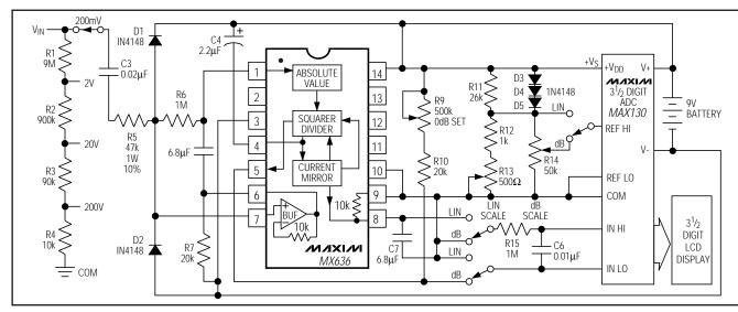
Figure 13. Portable High-Z Input RMS DPM and dB Meter
