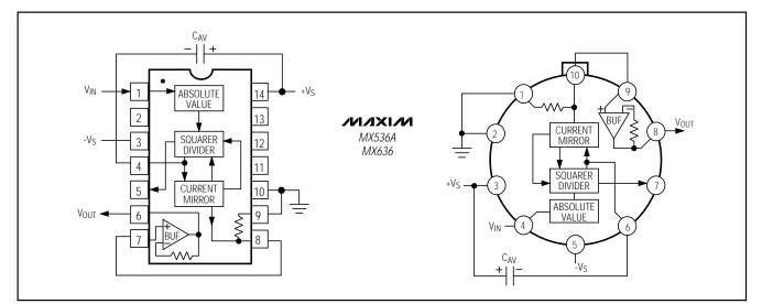
Figure 2. MX536A/MX636 Standard RMS Connection
