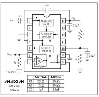
Figure 5. Single-Supply Operation
