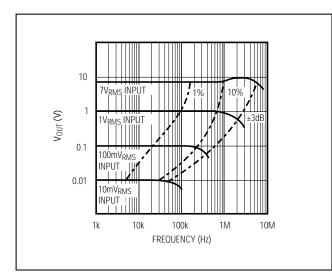
Figure 11. MX536A High-Frequency Response
