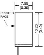
Dimensions are in mm (inch) Pin Tolerance:  $\pm 0.16$ mm(0.004 inch) Case Tolerance:  $\pm 0.25$  mm(0.01 inch)
