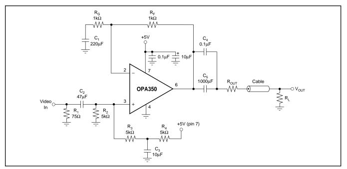
FIGURE 6. Single-Supply Video Line Driver.
