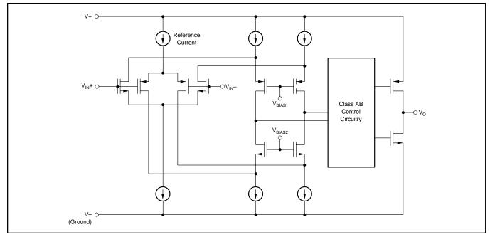
FIGURE 2. Simplified Schematic.
