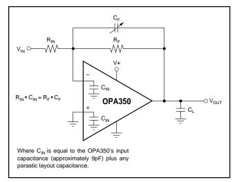
FIGURE 4. Feedback Capacitor Improves Dynamic Performance.
