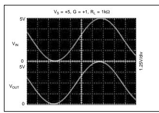
FIGURE 1. Rail-to-Rail Input and Output.
