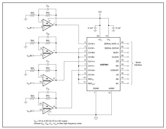
FIGURE 5. OPA4350 Driving Sampling A/D Converter.
