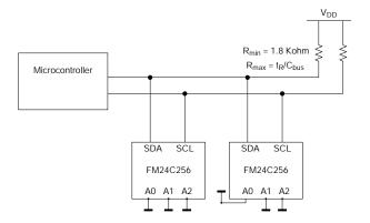
**Figure 2. Typical System Configuration**
