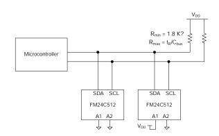
Figure 2. Typical System Configuration
