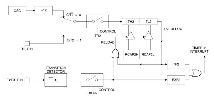
Figure 2. Timer 2 Auto Reload Mode (DCEN = 0)
