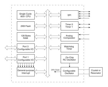
Figure 4-2. AT89LP214 Block Diagram
