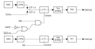
Note: RH0/RL0 are not required by Timer 0 during Mode 3 and may be used as temporary storage registers.
