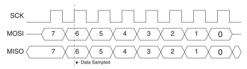
Figure 23-10. Serial Programming Interface Timing
