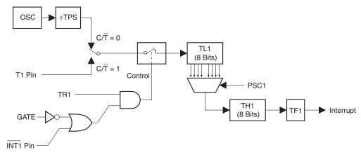
Mode 0 operation is the same for Timer 0 as for Timer 1, except that TR0, TF0 and  $\overline{\text{INT0}}$  replace the corresponding Timer 1 signals in Figure 14-1. There are two different GATE bits, one for Timer 1 (TMOD.7) and one for Timer 0 (TMOD.3). The  $\overline{\text{INT0}}$  and  $\overline{\text{INT1}}$  pins are shared with the XTAL oscillator. They may only be used for the GATE function when using the internal RC oscillator as the system clock.
