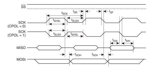
Figure 24-2. SPI Slave Timing (CPHA = 0)
