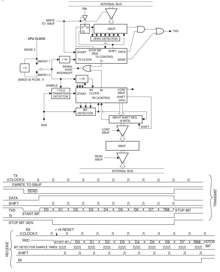
Figure 17-4. Serial Port Mode 3
