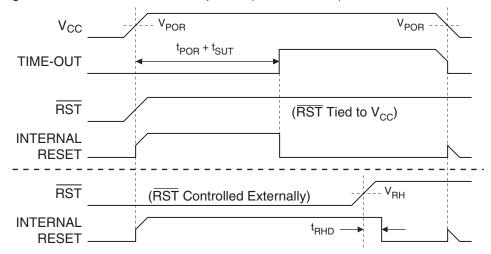
If the Brown-out Detector (BOD) is also enabled, the start-up timer does not begin counting until after  $V_{CC}$  reaches the BOD threshold voltage  $V_{BOD}$  as shown in Figure 10-2. However, if this event occurs prior to the end of the initialization sequence, the timer must first wait for that sequence to complete before counting.
