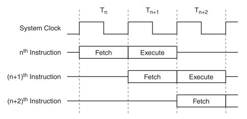
Figure 8-2. Single-cycle ALU Operation (Example: INC R0)
