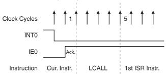
Figure 12-2. Maximum Interrupt Response Time
