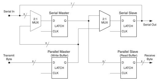
Figure 18-3. SPI Block Diagram
