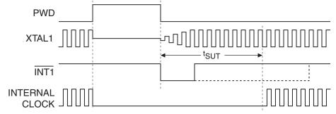
When PWDEX = "1", the wake-up period is controlled externally by the interrupt. Again, at the falling edge on the interrupt pin, power-down is exited and the oscillator is restarted. However, the internal clock will not propagate until the rising edge of the interrupt pin as shown in Figure 11-2. The interrupt pin should be held low long enough for the selected clock source to stabilize. After the rising edge on the pin the interrupt service routine will be executed.
