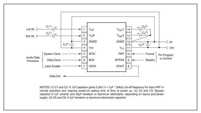
FIGURE 6. Typical Circuit Connection.
