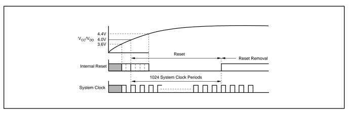
FIGURE 3. Internal Power-On Reset Timing.
