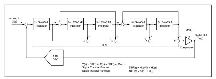
FIGURE 1. Simplified Diagram of the PCM1801 5th-Order Delta-Sigma Modulator.
