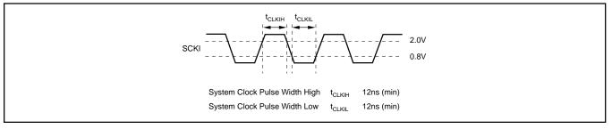
FIGURE 2. System Clock Timing.
