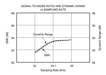
At  $T_A$  = +25°C, +V<sub>DD</sub> = +V<sub>CC</sub> = +5V,  $f_S$  = 44.1kHz, and SYSCLK = 384 $f_S$ , unless otherwise noted.
