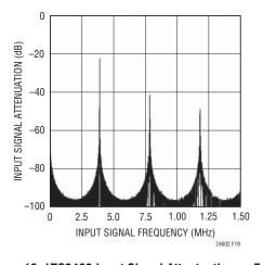
Figure 19. LTC2462 Input Signal Attentuation vs Frequency
