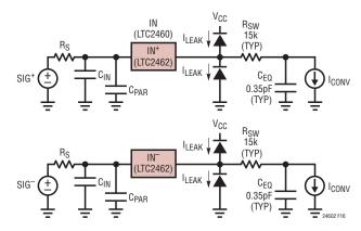
Figure 16. LTC2460/LTC2462 Input Drive Equivalent Circuit
