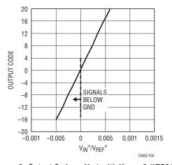
Figure 3. Output Code vs  $V_{IN}^+$  with  $V_{IN}^- = 0$  (LTC2462)
