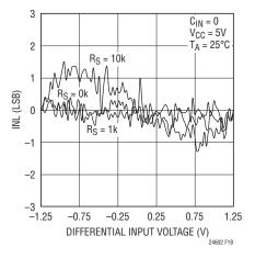
Figure 18. Measured INL vs Input Voltage
