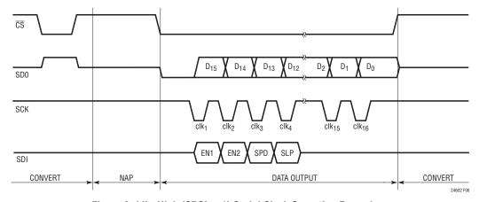
Figure 6. Idle-High (CPOL = 1) Serial Clock Operation Example. The Rising Edge of  $\overline{\text{CS}}$  Starts a New Conversion
