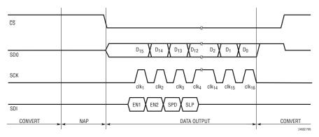
Figure 9. Idle-Low (CPOL = 0) Clock. The 16th SCK Falling Edge Triggers a New Conversion
