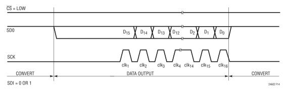
Figure 14. 2-Wire, Idle-Low (CPOL = 0) Serial Clock Operation Example
