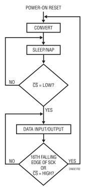
Figure 2. LTC2460/LTC2462 State Transition Diagram
