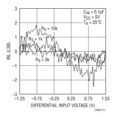
Figure 17. Measured INL vs Input Voltage
