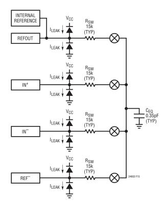
Figure 15. LTC2460/LTC2462 Analog Input/Reference Equivalent Circuit
