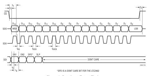
Figure 4. Data Input/Output Timing
