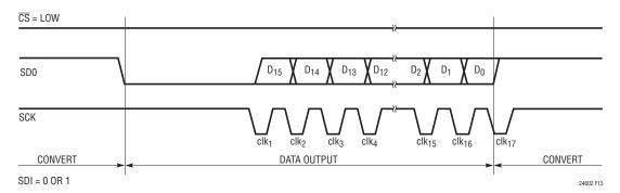
Figure 13. 2-Wire, Idle-High (CPOL = 1) Serial Clock, Operation Example
