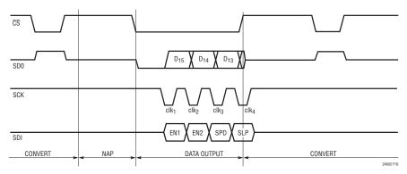
Figure 10. Idle-High (CPOL = 1) Clock and Aborted I/O Example
