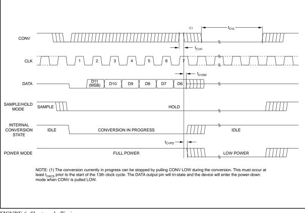
FIGURE 6. Short-cycle Timing.
