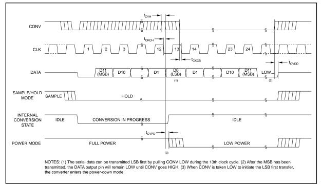
FIGURE 5. Serial Data "LSB-First" Timing.
