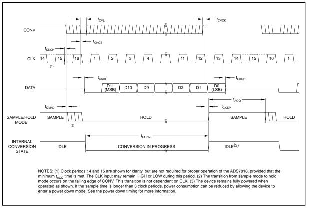
FIGURE 3. Basic Conversion Timing.
