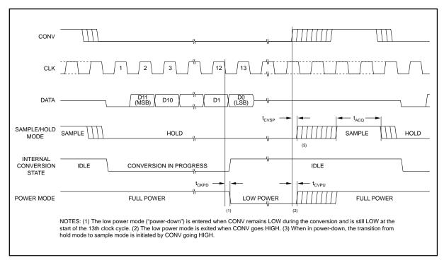
FIGURE 4. Power-down Timing.
