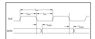
FIGURE 2. Serial Data and Clock Timing.
