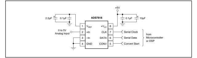
FIGURE 1. Basic Operation of the ADS7818.
