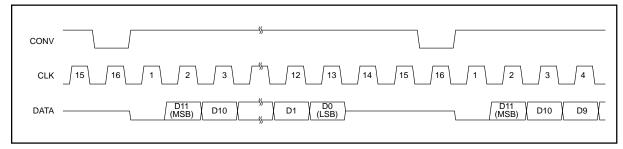
FIGURE 8. Typical DSP Interface Timing.
