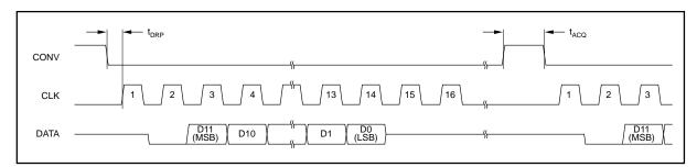
FIGURE 9. Typical SPI/QSPI Interface Timing.
